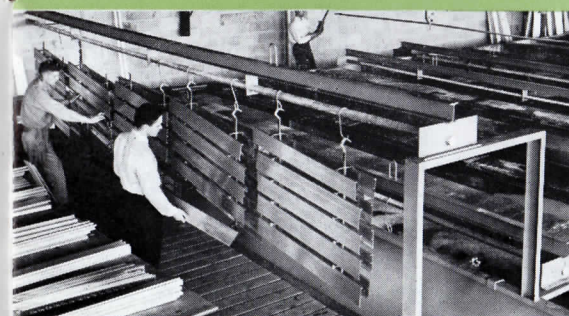
Fifty extruded aluminum slats are racked in dip assembly at a time to begin processing on the Architectural Aluminum Alodizing line.
