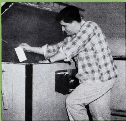
NATE GIORGIO, Laboratory Technician, working at the salt spray tank in our Quality Control Center.
