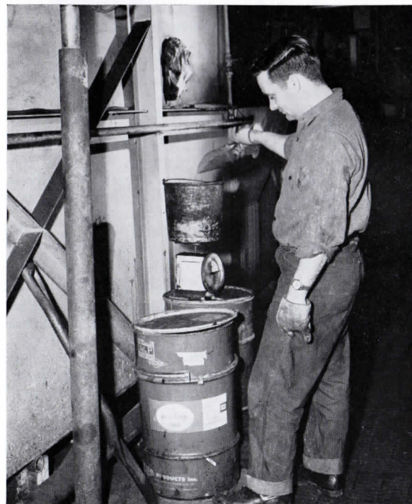
Quantity of Alodine used in process is measured from drum.
