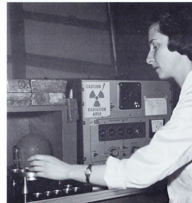
(E.) RADIOISOTOPE COUNTER. This modern device detects radioactivity in any radioactive substance, such as compounds containing Carbon 14 and tritium.
