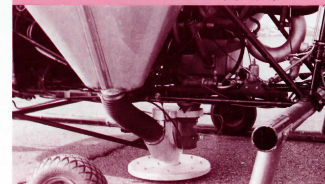
Close-up of first mounting of Amchem centrifugal sprayer rig on TVA helicopter at Muscle Shoals. Picture was taken on March 15.
