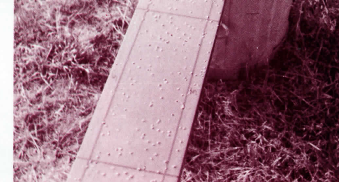
Calibration method used in determining amount and distribution of Aqua Kleen granules when applied with Amchem's new centrifugal sprayer.
