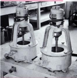
Centrifuges where syrup and crystals are separated three times. The third stage takes place when no crystals but only molasses remains.
