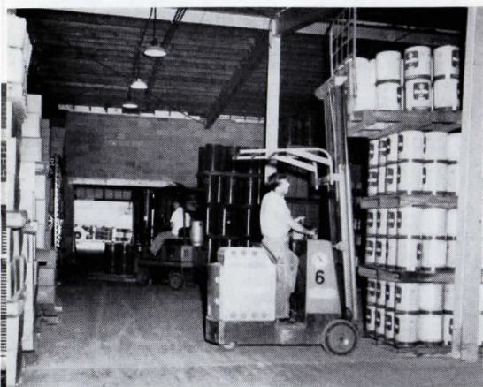
BOB LEAHY deftly glides his fork lift truck into position to stack a pallet of Weed Killer 66. Note how steel overhead canopy and grill on forklift protect Bob in case of slip-page, thus eliminating accident hazard.
