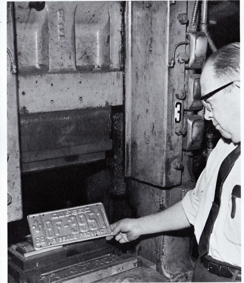
Some resident of Quebec will eventually display this license plate on his automobile. Plate has just been embossed by 75-ton pressure press—one of five at the Morin plant in Montmagny. Donat Morin gives it the once over.
