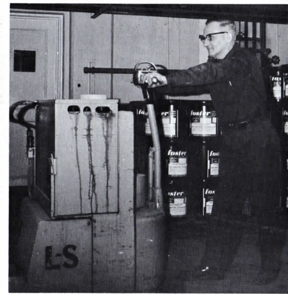
Melvin Kratz operates jack stacker that has lifting capacity of 2,000 pounds.
