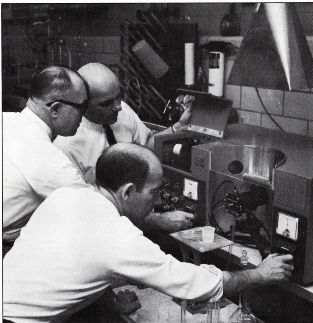
Chief analytical chemist Lou Sabatini with chemists Don McKeever and Warren Snyder (counterclockwise) are adjusting the controls on the spectrophotometer to attain its maximum sensitivity prior to making a waste water sample analysis. This new Perkin-Elmer Atomic Absorption Spectrophotometer electronically measures contaminants in quantities of less than one part per million. According to Sabatini's explanation, the spectrophotometer functions as follows: A liquid sample is aspirated (carried or projected) into a flame. The flame-dissociated (or separated) atoms absorb radiant energy emitted by a hollow cathode tube which is specific for the particular element being sought. Comparison is then made, by a detector, of the total energy radiated by the tube with the total energy less the amount absorbed by the atoms of the element being determined. The results are revealed to the analyst on a digital readout system. With this information, the analyst is able to compute ppm (parts per million) of an element in a sample submitted for analysis.
