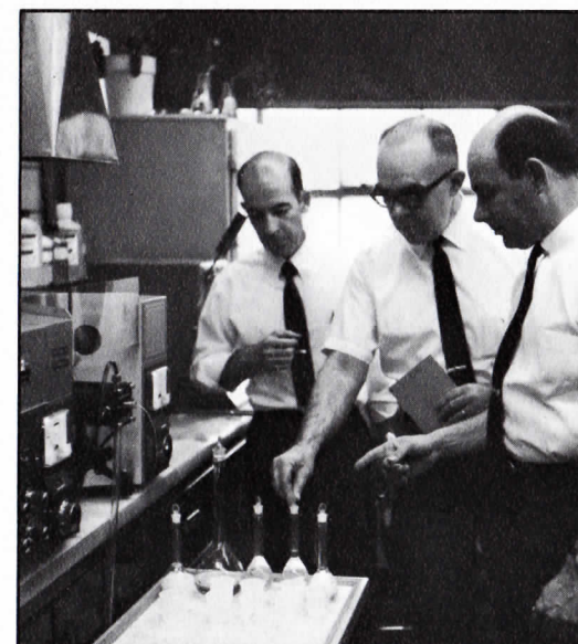
In conjunction with an assignment from Amchem's Hydro-Fax Division, Analytical chemists Snyder, McKeever, and Sabatini (left to right) are performing quantitative analyses of waste water samples before and after these samples had been treated for removal of contaminants. Analyses were made on the atomic absorption spectrophotometer (shown at left) which was recently installed in Lab 4.
