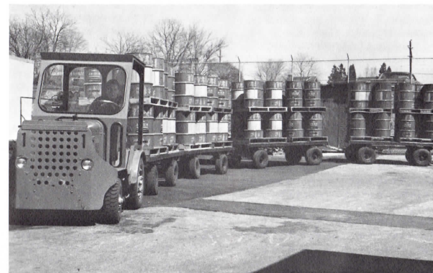
By using a tandem of flat cars and double-deck stacking the filled drums, one truck operator can move over eight times as many drums as one tork lift truck.
