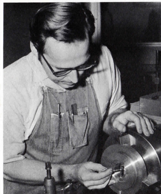
Jerry Barba machining plate housing for Microfoil pump.
