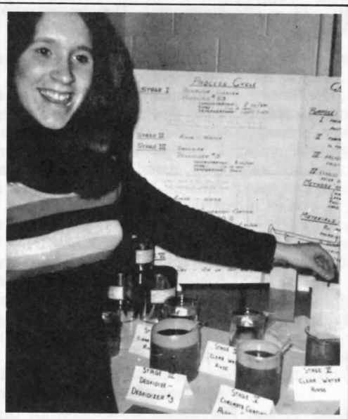
Karen dips an aluminum test panel in a final rinse, the sixth stage, of an Alodine® pre-paint treatment in a demonstration for the judges.
