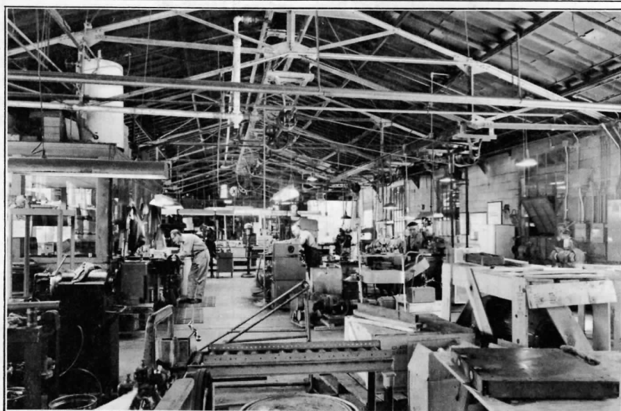
(Above, left) Maintenance shop before removal of overhead power belts. (At right) Machinist Charlie Jones operates new, direct-power milling machine.
