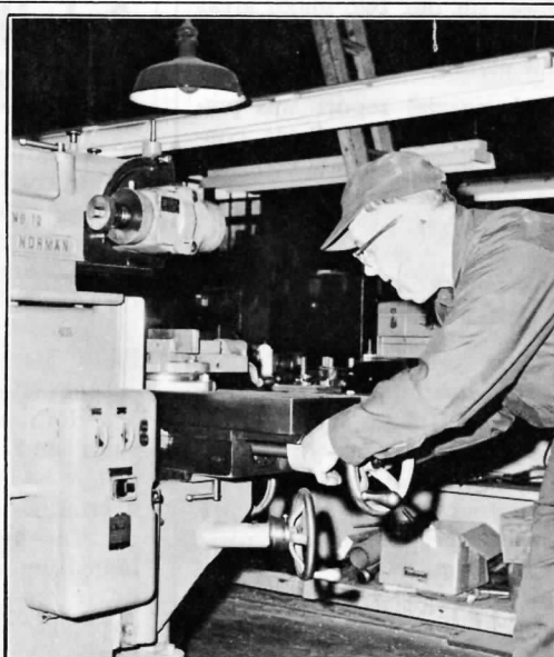
(Above, left) Maintenance shop before removal of overhead power belts. (At right) Machinist Charlie Jones operates new, direct-power milling machine.
