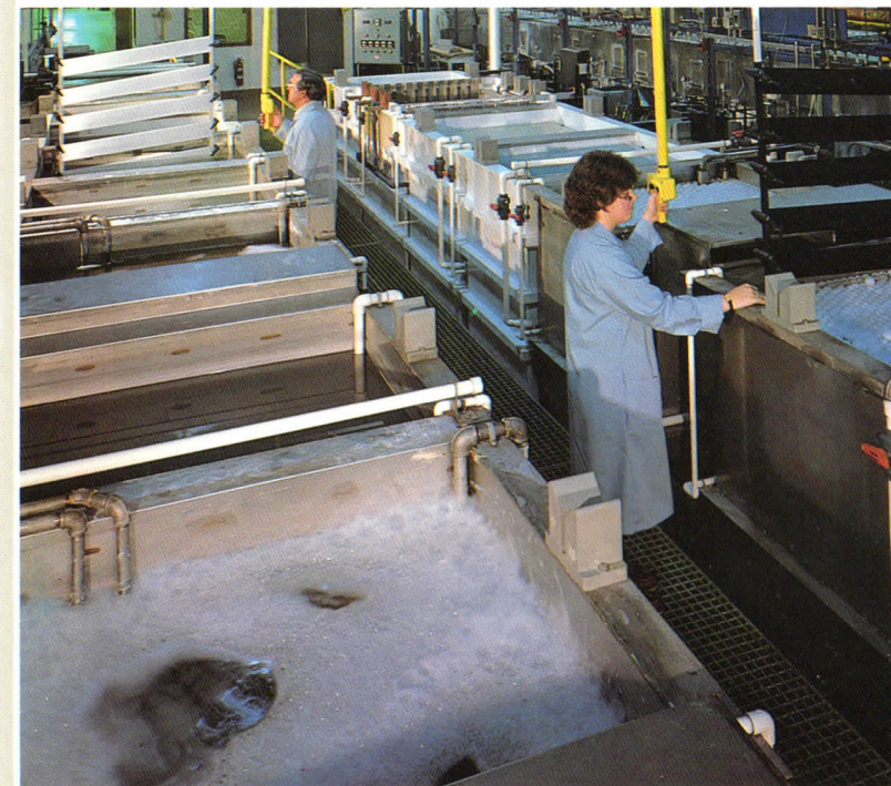
Technicians process aluminum extrusions on pilot anodizing line
